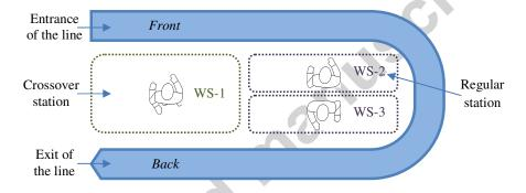
Figure 1. Typical illustration of a U-shaped line configuration
