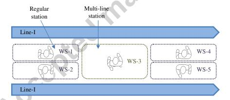
Figure 2. Schematic view of a parallel line system
