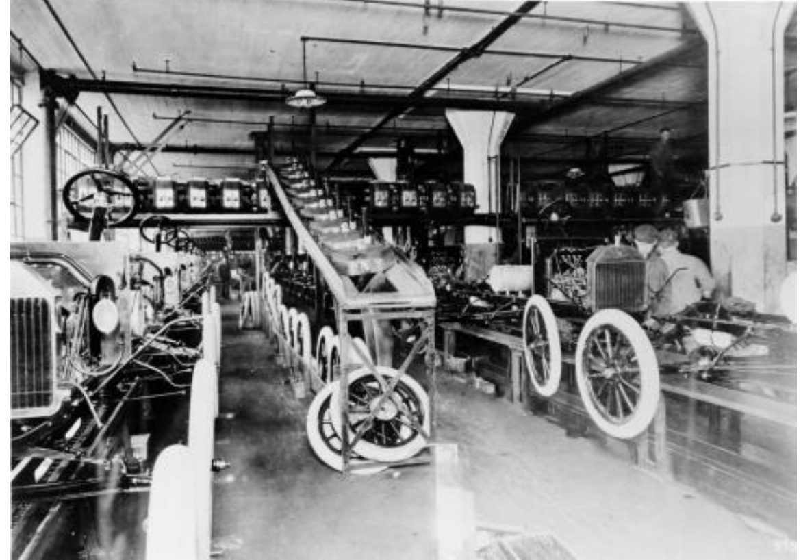
Highland Park'ta Ford'un Unlu T-Modelinin Montajı ( media.ford.com/content/fordmedia )
