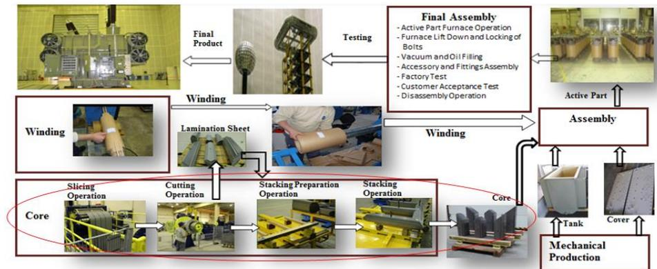
Fig. 5: Summarized production flow chart for magnetic core production.
